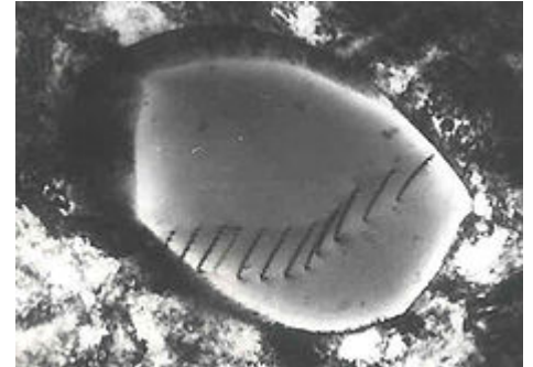
Transmission electron micrograph of dislocations in steel, which are faults in the structure of the crystal lattice at the atomic scale
