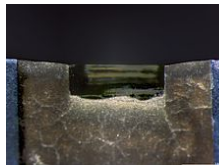
A diamond knife blade used for cutting ultrathin sections (typically 70 to 350 nm) for transmission electron microscopy.
